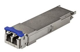
The QSFP40GLR4ES is a Dell EMC QSFP-40G-LR4 compatible fiber transceiver module that has been designed, programmed and tested to work with Dell EMC brand switches and routers. It delivers dependable 40 GbE connectivity over fiber cable, for 40GBase-LR4 compliant networks, with a maximum distance of up to 10 km (6.2 mi).
