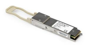
The QSFP-40G-ESR4-ST is an MSA compatible fiber transceiver module that has been designed, programmed and tested to work with MSA brand switches and routers. It delivers dependable 40 GbE connectivity over fiber cable, for 40GBase-SR4 compliant networks, with a maximum distance of up to 300 m (984 ft).
