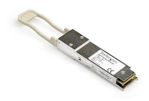
The QSFP-40G-CSR4-ST is a Cisco QSFP-40G-CSR4 compatible fiber transceiver module that has been designed, programmed and tested to work with Arista Networks brand switches and routers. It delivers dependable 40 GbE connectivity over fiber cable, for 40GBase-SR4 compliant networks, with a maximum distance of up to 400 m (1312 ft.).
