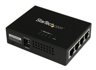
This Gigabit midspan PoE+ injector is a cost-effective alternative to upgrading your existing network switch to a PoE-capable model.
