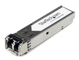
The PLUS-SR-ST is a Palo Alto Networks PAN-SFP-PLUS-SR compatible fiber transceiver module that has been designed, programmed and tested to work with Palo Alto Networks brand switches and routers. It delivers dependable 10 GbE connectivity over fiber cable, for 10GBase-SR compliant networks, with a maximum distance of up to 300 m (984 ft).
