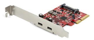
This PCIe USB 3.1 Gen 2 card installs into an available PCI-Express slot in your computer and enables you to upgrade your current system by adding two USB-C (10Gbps) ports.
