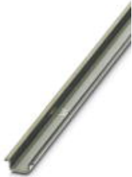
DIN rail, material: Steel, unperforated, height 5.5 mm, width 15 mm, length: 2 m
