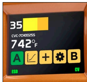
Tip temperature displayed on large color screen.
