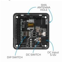
COM GSM RXD/TXD can be connected to M5Stack's UART (TX(0/13/17)RX(5/15/16)) by setting the DIP switch. Since these GPIO in **M5Stack Fire** 16/17 are connected to PSRAM by default, conflicts may occur when using GSM. It is recommended to use any set of UART pins in the remaining two groups.
