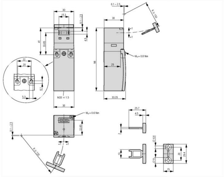
Switch must not be used as a mechanical stop Terminal marking according to EN 50 013 Travel [mm] = Contact closed = Contact open Zw = Positive opening sequence
