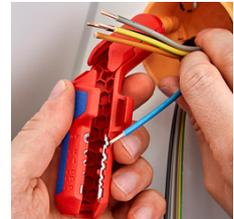
Wire stripping on single conductors
