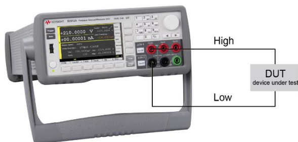
Same measurement using an SMU
