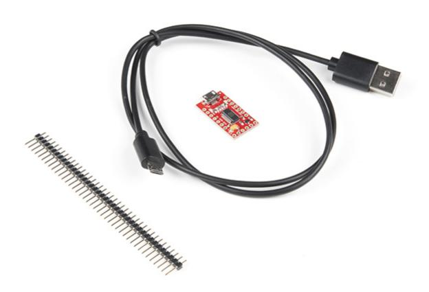
The SparkFun FT231X Breakout Kit provides you with everything that you need to get started with FTDI with the full UART hardware handshake feature! The pin-out of the included FT231X Breakout board matches the FTDI cable to work with official Arduino and cloned Arduino boards. It can also be used for general serial applications.
