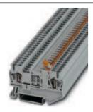
Knife disconnect terminal block, Connection type: Spring-cage connection, Cross section: 0.08 mm² - 4 mm², AWG: 28 - 12, Nominal current: 20 A, Nominal voltage: 400 V, Length: 60.5 mm, Width: 5.2 mm, Color: gray, Assembly: NS 35/7,5, NS 35/15
