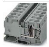
Feed-through terminal block, Connection method: Spring-cage connection, Cross section: 2.5 mm² - 35 mm², AWG: 14 - 2, Width: 16 mm, Color: gray, Mounting type: NS 35/7,5, NS 35/15
