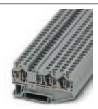
Feed-through terminal block, Connection method: Spring-cage connection, Cross section: 0.08 mm² - 6 mm², AWG: 28 - 10, Width: 6.2 mm, Color: gray, Mounting type: NS 35/7,5, NS 35/15
