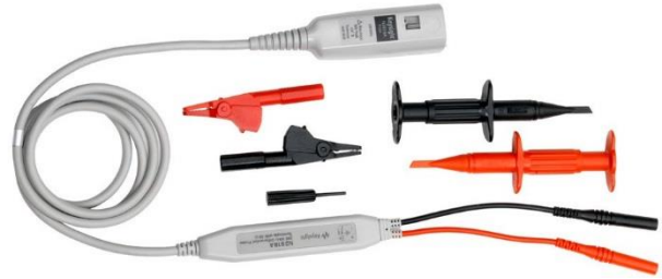
Figure 13. Keysight's N2818A 200-MHz differential active probe.
