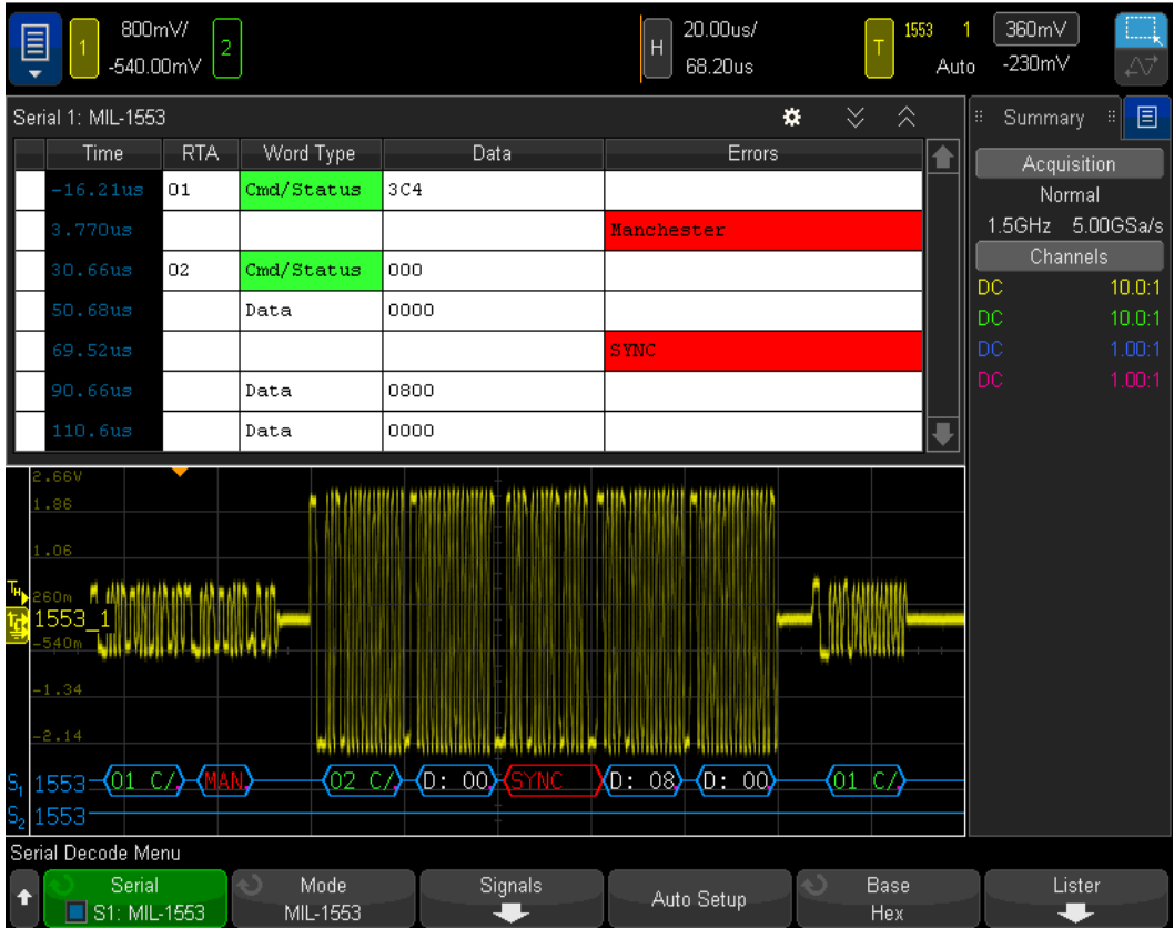
Figure 2. MIL-STD 1553 decode on an InfiniiVision X-Series oscilloscope.
