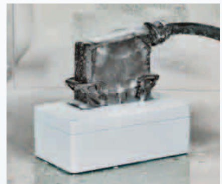
HEAVYCON EVO plug-in connector in the climatic chamber at -50°C
