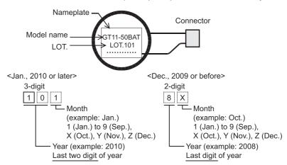
The production date of the battery built in the purchased GOT can be confirmed by the production No. (S/N) marked on the GOT main unit.
