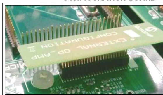
FIGURE 2: EXTERNAL OP AMP CONFIGURATION BOARD
