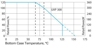
Derating (thermal resist.) UXP 300: 4.35 W/°K (0.23°K/W) Power rating: 300 W at 85°C bottom case temp.\* Please ask for detailed mounting procedure!
