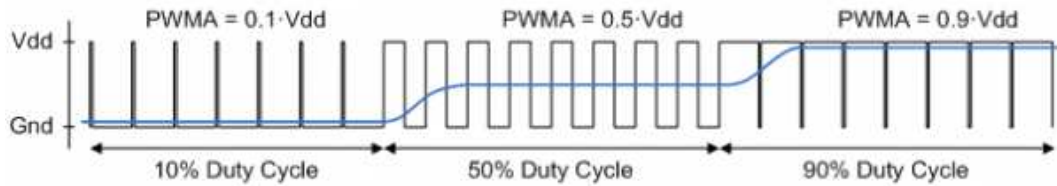
( https://reference.digilentinc.com/_detail/reference/programmable-logic/nexys-a7/n4ah.png?id=reference%3Aprogrammable-logic%3Anexys-a7%3Areference-manual ) Figure 15.1.2 Representation of a PWM Integrator Producing an Output Voltage by Integrating the Pulse Train
