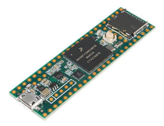
The Teensy is a breadboard-friendly development board with loads of features in a tiny package. Each Teensy 3.6 comes with headers already attached and pre-flashed with a bootloader so you can program it using the on-board USB connection; no external programmer needed! You can program for the Teensy in your favourite program editor using C or you can install the Teensyduino add-on for the Arduino IDE and write Arduino sketches for it!
