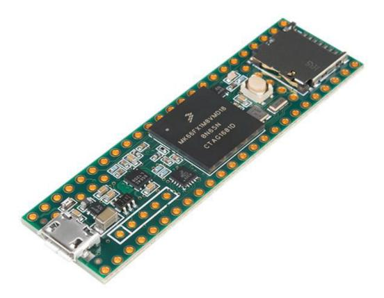
The Teensy is a breadboard-friendly development board with loads of features in a tiny package. Each Teensy 3.6 comes pre-flashed with a bootloader so you can program it using the on-board USB connection; no external programmer needed! You can program for the Teensy in your favourite program editor using C or you can install the Teensyduino add-on for the Arduino IDE and write Arduino sketches for it!
