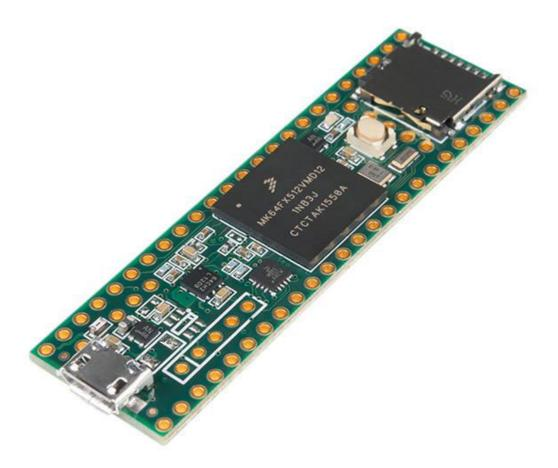
The Teensy is a breadboard-friendly development board with loads of features in a tiny package. Each Teensy 3.5 comes pre-flashed with a bootloader so you can program it using the on-board USB connection: no external programmer needed! You can program for the Teensy in your favourite program editor using C or you can install the Teensyduino add-on for the Arduino IDE and write Arduino sketches for it!
