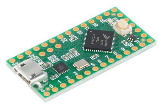
The Teensy is a breadboard-friendly development board with loads of features in a tiny package. The Teensy LC (Low Cost) is a 32 bit microcontroller board that provides you with an uncomplicated option for getting started with the Teensy line of products without breaking the bank!
