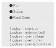
The LEDs on the front of the Variable Speed Starter indicate operating status and faults
