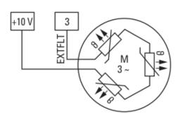
Depending on the configuration of the input terminals the function "external fault" (EXTFLT) is assigned to terminal 3. This Input can also be used to connect a thermistor. Wiring see picture on the left hand side.
