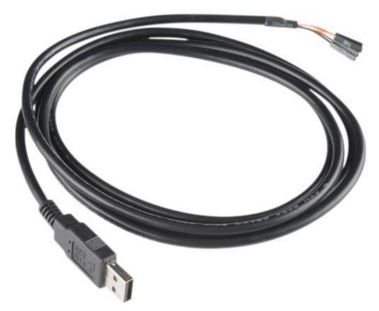
This is a USB to TTL Serial Cable which allows for a simple way to connect TTL interface devices to USB. The I/O pins of this cable are configured to operate at 3.3V specifically with a Raspberry Pi with each serial pin broken apart. Thanks to its separated pins, this cable is a perfect candidate for powering, connecting, and accessing the login and debug console on the Raspberry Pi.
