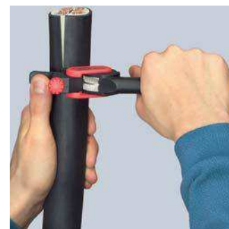
Turning the tool for circumferential cut
