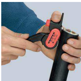
Setting the tool for longitudinal cut
