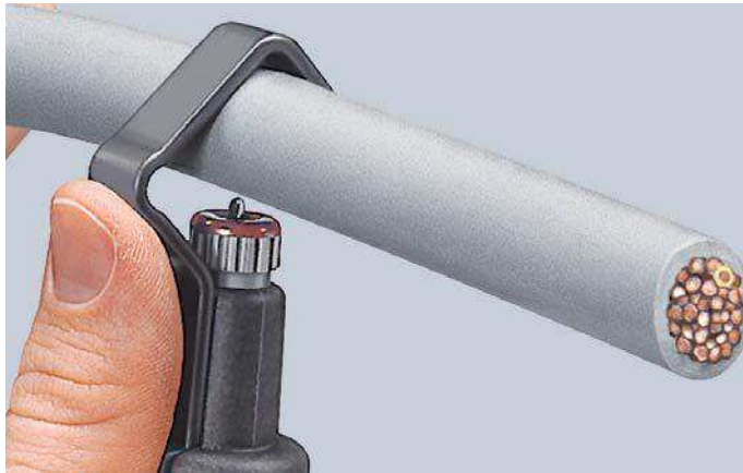
Setting the tool for circular cutting
