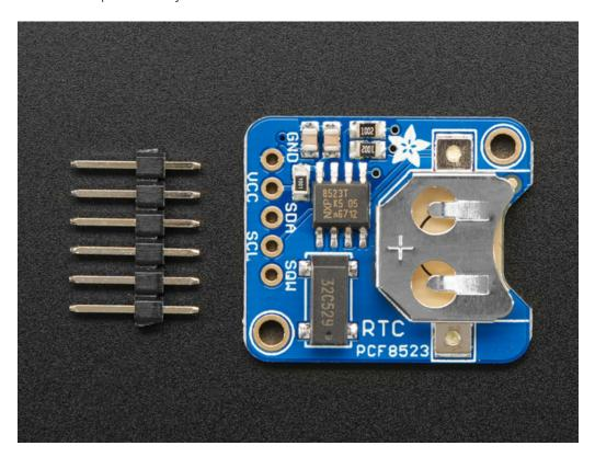
The PCF8523 is simple and inexpensive but not a high precision device. It may lose or gain up to 2 seconds a day. For a high-precision, temperature compensated alternative, please check out the DS3231 precision RTC (http://adafru.it/3013). If you need a DS1307 for compatibility reasons, check out our DS1307 RTC breakout (http://adafru.it/3296)
