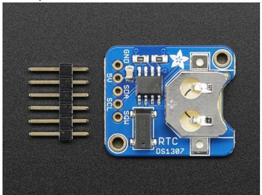
Assembly is really easy, you can use straight or 'right-angle' style headers to attach to the PCB. We'll be using the plain straight headers included
