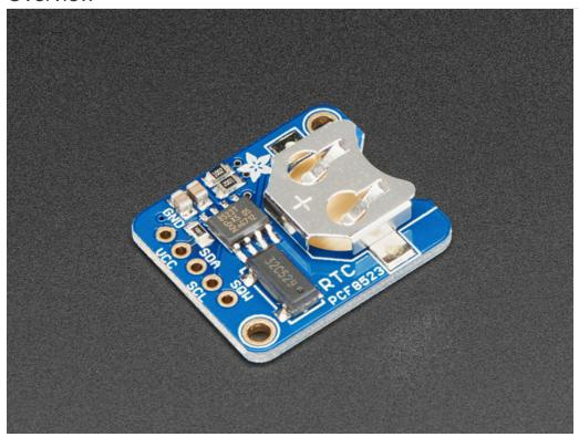
This is a great battery-backed real time clock (RTC) that allows your microcontroller project to keep track of time even if it is reprogrammed, or if the power is lost. Perfect for datalogging, clock-building, time stamping, timers and alarms, etc. Equipped with **PCF8523** RTC - it can run from 3.3V *or* 5V power & logic!
