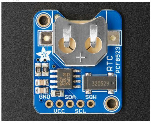
The PCF8523 is a I2C device. That means it uses the two I2C data/clock wires available on most microcontrollers, and can share those pins with other sensors as long as they don't have an address collision.
