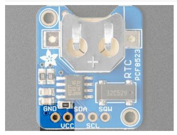
VCC - this is the power pin. This chip can be powered by 3-5VDC so there is now on-board regulator. To power the board, give it the same power as the logic level of your microcontroller - e.g. for a 5V micro like Arduino, use 5V
