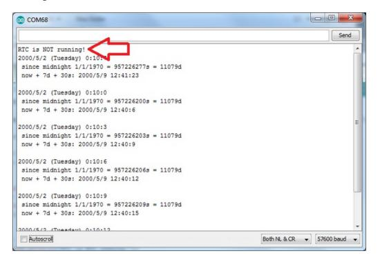
Whenever the RTC chip loses all power (including the backup battery) it will reset to an earlier date and report the time as 0:0:0 or similar. Whenever you set the time, this will kickstart the clock ticking.
