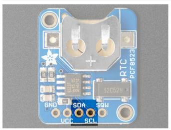
**SCL** - I2C clock pin, connect to your microcontrollers I2C clock line.
