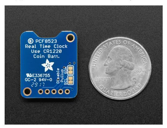
Works great with an Arduino using our RTC library (https://adafru.it/c7r) or with a Raspberry Pi (or similar single board linux computer) (https://adafru.it/C5q)
