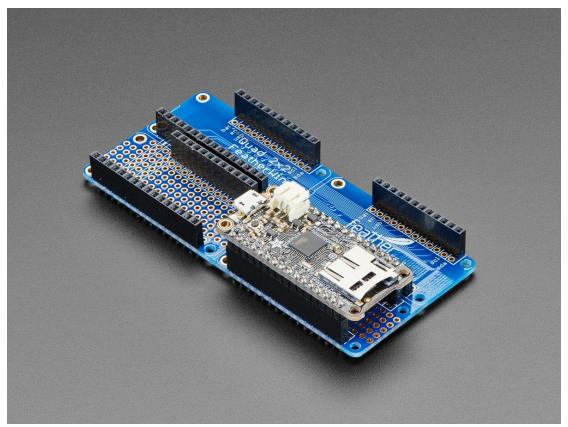
This is the FeatherWing Quad 2x2 – a prototyping add-on and more for all Feather boards. This is similar to a FeatherWing Proto except there are four! The magic of the Quad comes when you want to connect your Feather to three other Feather Wings without needing any stacking headers. The boards are all set up in a 2x2 grid.
