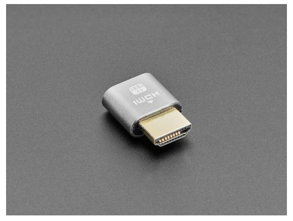
This HDMI Dummy Plug is a small device that acts as a display emulator. Once it's plugged into the video output socket on your device or computer, the plug fools the operating system into detecting a connected display, and then you have unimpeded access to your graphics card hardware.
