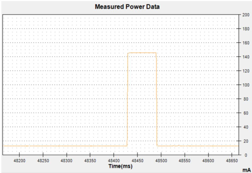
The ~13mA quiescent current is the current draw for listening (~2mA) plus ~11mA for the microcontroller. This can be reduced to almost nothing with proper sleep modes and not putting the module in active listen mode!
