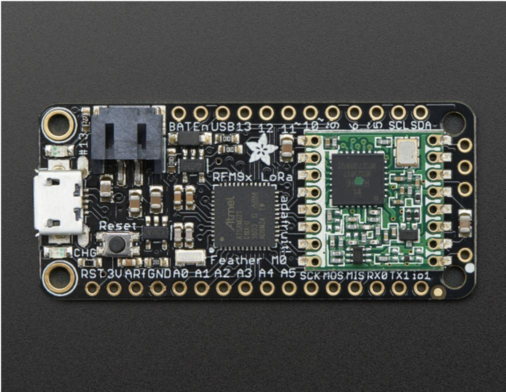
At the Feather M0's heart is an ATSAM21G18 ARM Cortex M0 processor, clocked at 48 MHz and at 3.3V logic, the same one used in the new [Arduino Zero](#). This chip has a whopping 256K of FLASH (8x more than the Atmega328 or 32u4) and 32K of RAM (16x as much)! This chip comes with built in USB so it has USB-to-Serial program & debug capability built in with no need for an FTDI-like chip.
