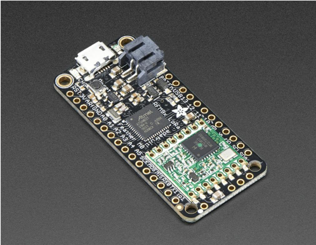
This is the **Adafruit Feather M0 RFM95 LoRa Radio (433 or 900 MHz)** - our take on an microcontroller with a "[Long Range \(LoRa\)](#)" packet radio transceiver with built in USB and battery charging. Its an Adafruit Feather M0 with a Long Range radio module cooked in! Great for making wireless networks that are more flexible than Bluetooth LE and without the high power requirements of WiFi. [We have other boards in the Feather family, check'em out here.](#)
