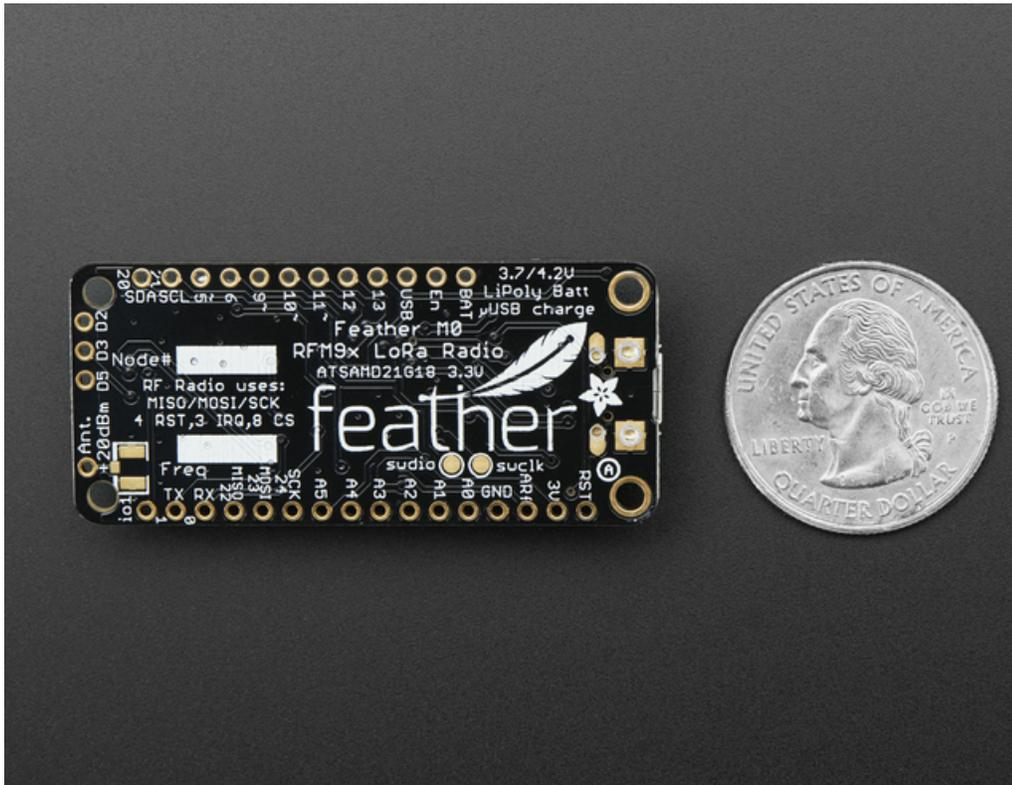
This **Feather M0 LoRa Radio** uses the extra space left over to add an RFM9x LoRa 868/915 MHz radio module. These radios are not good for transmitting audio or video, but they do work quite well for small data packet transmission when you need more range than 2.4 GHz (BT, BLE, WiFi, ZigBee).
