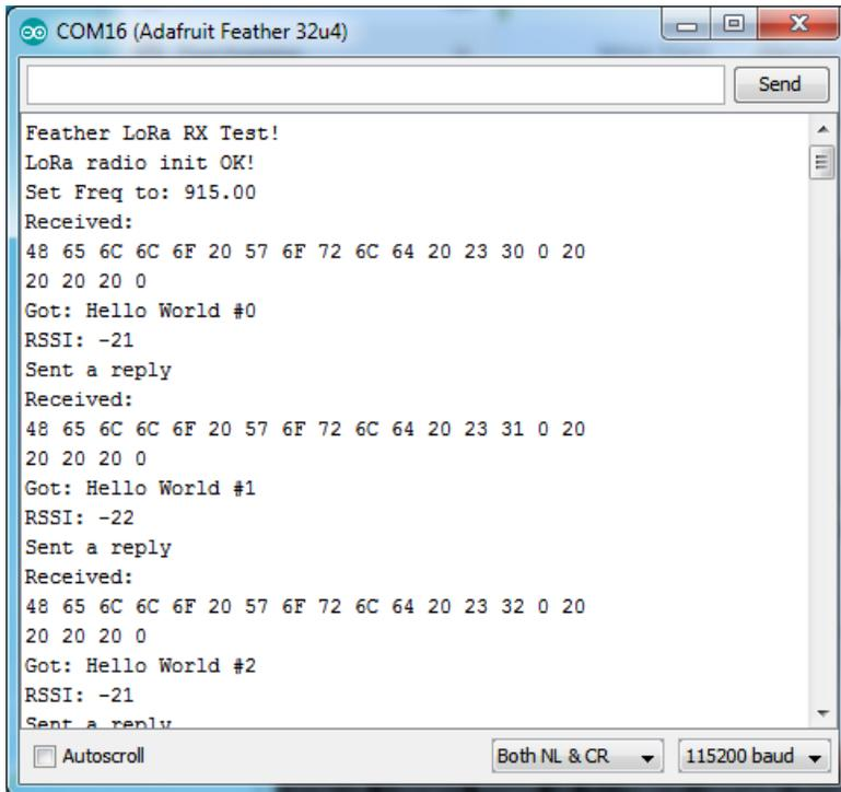
You can see that the library example prints out the hex-bytes received `48 65 6C 6C 6F 20 57 6F 72 6C 64 20 23 30 0 20 20 20 0`, as well as the ASCII 'string' `Hello World`. Then it will send a reply.
