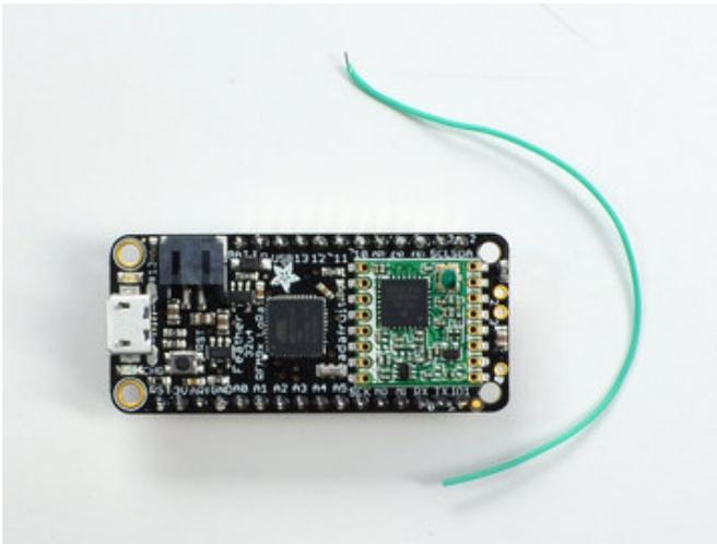
Cut a stranded or solid core wire to the proper length for the module/frequency
