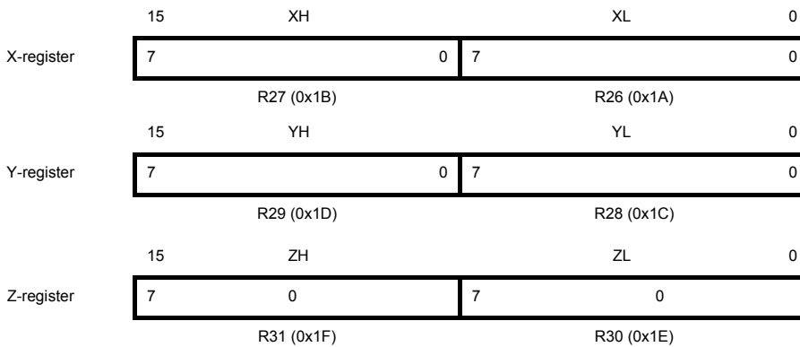
Figure 11-3. The X-, Y- and Z-Registers
