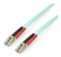
The A50FBLCLC5 5m 850nm Laser-Optimized Multimode Fiber (LOMMF) Aqua Cord features 50/125 micron fiber for high-speed, high bandwidth data transmissions over 10 Gigabit Ethernet and Fiber Channel networks - the perfect solution for fiber cable runs between multiple backbone switches, hubs and routers as well as higher end networking equipment.
