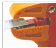
Ideal for flat cable stripping
