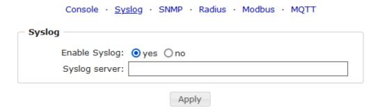
Enable Syslog: Enables the usage of Syslog Messages.
