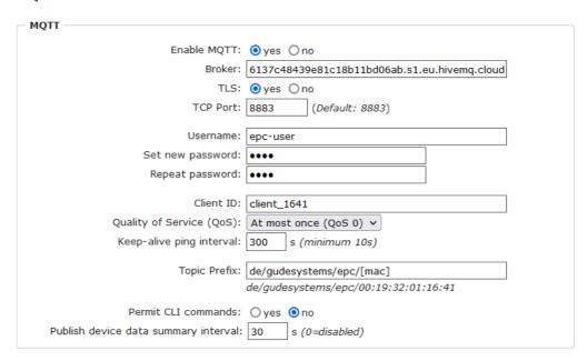
Enable MQTT: Enables MQTT support.
