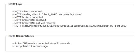
MQTT Logs: Outputs individual log messages about the connection setup.
