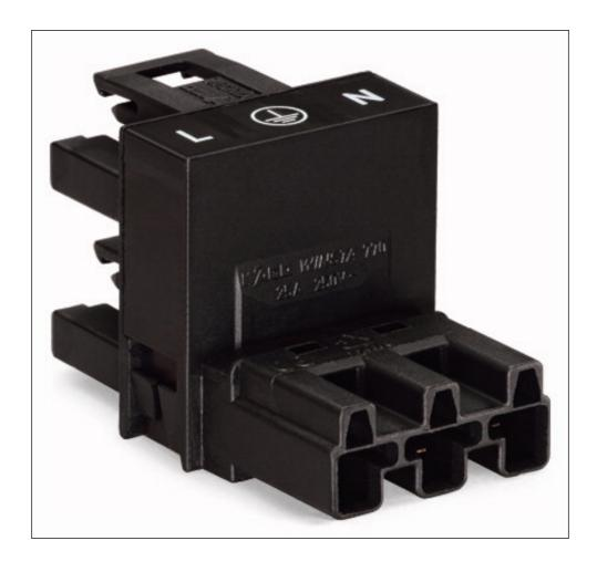
Printview: h-distribution connector; 1 x plug / 2 x socket; 3-pole; for "flying leads"; with 3rd locking lever; 100% protected against mismating; pluggable - Item No.: 770-936
