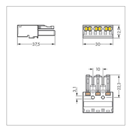
Printview: Socket; without strain relief housing; 3-pole; 100% protected against mismating; 2-conductor connection; Pin spacing 10 mm / 0.394 in - Item No.: 770-1303
