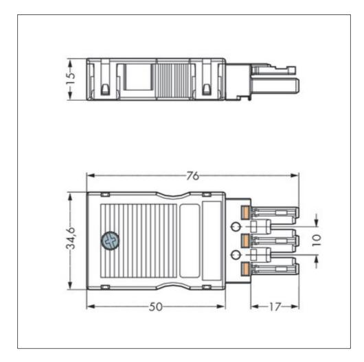
Printview: Socket; with strain relief housing; 3-pole; Pin spacing 10 mm / 0.394 in; 100% protected against mismating; Cable diameter 8 - 11.5 mm - Item No.: 770-103
