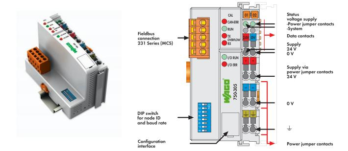
This buscoupler connects the WAGO-I/O-SYSTEM as a slave to the CAL field-bus. The module data is transmitted using Communication Objects (COB).
