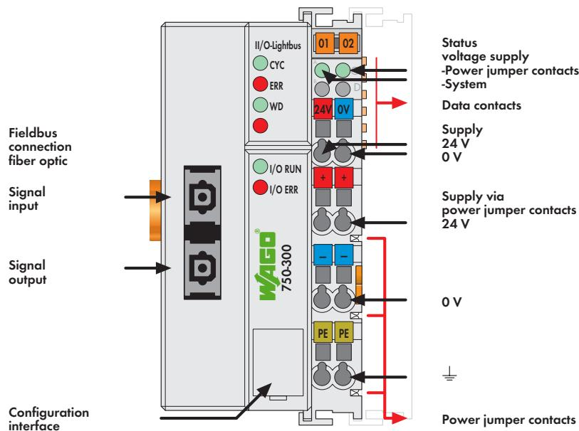
This buscoupler connects the WAGO-I/O-SYSTEM as a slave to the LIGHTBUS fieldbus.
