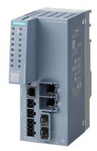
SCALANCE SC642-2C Cyber Security Appliance; For protection of devices and networks in discrete manufacturing and the process industry for protection of industrial communication with firewall and VPN; Further functions: address translation (NAT/NAPT); Connection to SINEMA RC; 2x combo port electrical or optical; 10/100/1000 Mbps RJ45 or 100 Mbps SFP or 1000 Mbps SFP
