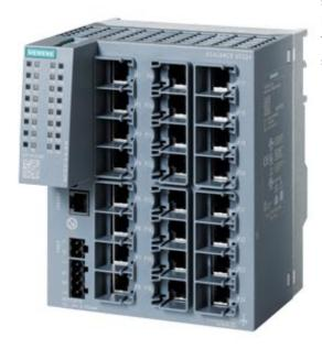
SCALANCE XC224 manageable layer 2 IE Switch; 24x 10/100 Mbit/s RJ45-Ports; 1x console port, Diagnostic LED; Redundant power supply; Temp. range -40°C to +70 °C Mounting: Standard Mounting Rail/S7 Profile Rail/Wall Office redundancy functions features (RSTP, VLAN,...); PROFINET IO device Ethernet/IP-compliant, C-PLUG shaft.
