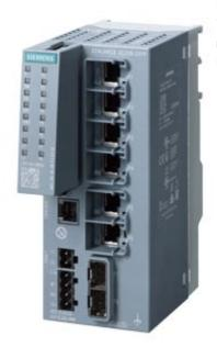
SCALANCE XC206-2SFP manageable layer 2 IE Switch; 6x 10/100 MBit/s RJ45 ports; 2x 100/1000 MBit/s SFP; 1x console port; Diagnostic LED; Redundant power supply; Temp. range -40°C to +70 °C Mounting: Standard Mounting Rail/S7 Profile Rail/Wall Office redundancy functions features (RSTP, VLAN ,...); PROFINET IO Device; Ethernet/IP compliance C-PLUG shaft;
