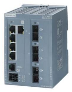
Preset for Ethernet/IP mode! SCALANCE XB205-3LD managed Layer 2 IE Switch 5x 10/100 Mbit/s RJ45 ports 3x MM FO SC port 1x console port, diagnostics LED redundant power supply; temp. range 0 °C to +60 °C; mounting onto standard rail; Default EtherNet/IP
