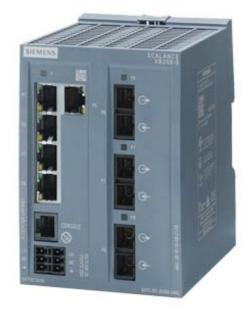
Preset for PROFINET mode! SCALANCE XB205-3 managed Layer 2 IE Switch 5x 10/100 Mbit/s RJ45 ports 3x MM FO SC port 1x console port, diagnostics LED redundant power supply; temp. range 0 °C to +60 °C; mounting onto standard rail; Default PROFINET
