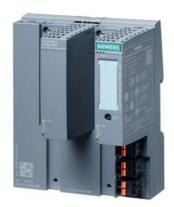
SCALANCE XF204-2BA managed IE switch, 4 x 10/100 Mbit/s, IEC 62443-4-2 certified; 2 x BusAdapter interface, error signaling contact, set pushbutton, redundant 24 V DC power supply, PROFINET device, extended temperature range -40  $^{\circ}$ C...+70  $^{\circ}$ C, conformal coating, with electr. manual on DVD, C-PLUG optional, supplied without BusAdapter
