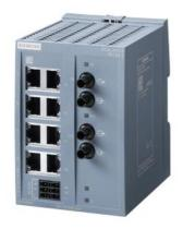
SCALANCE XB108-2 unmanaged IE switch, 8x 10/100 Mbit/s ports, 2x 100 Mbit/s multimode BFOC, for setting up small star and line topologies, LED diagnostics, IP20, redundant power supply 24 V AC/DC manual available as a download .
